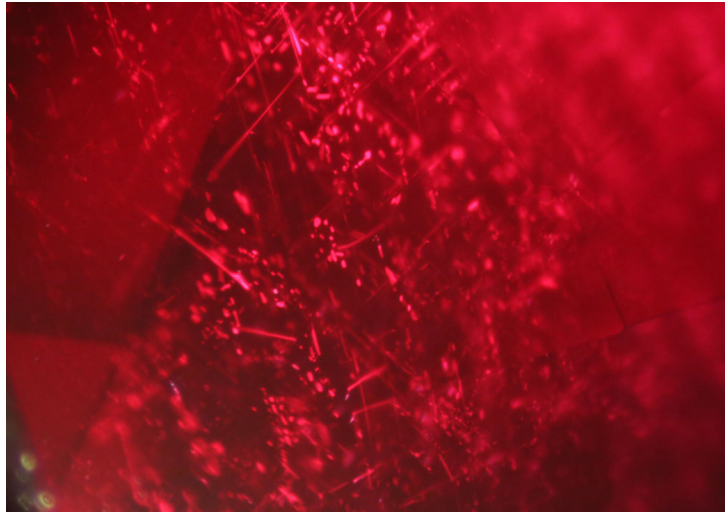
Rutile needles, platelets and particles oriented in three directions as seen in this 1.71 ct Mozambican ruby.
